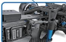
Carbon fiber upper deck provides two servo mounting options for adjustable weight balance.
