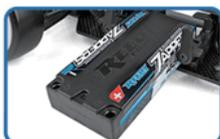
The motor position can be mounted high, and battery moved back for more rear weight bias.
